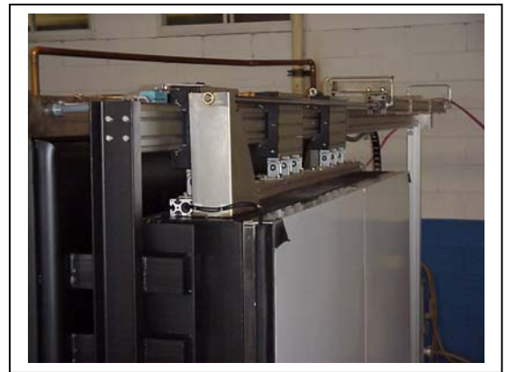
Horizontal sliding door slide assembly & pneumatic cylinder
