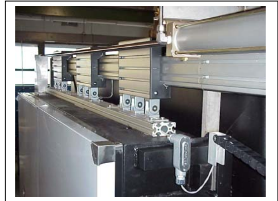
Horizontal sliding door slide assembly & pneumatic cylinder
