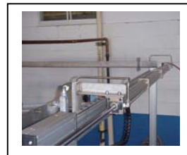
Pneumatic cylinder & support post
