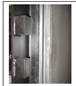
Door retaining block & gasket in machined groove
