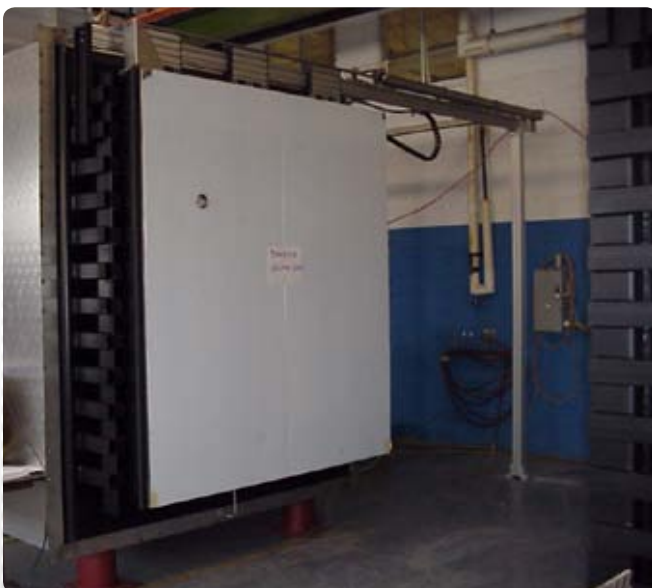
Horizontal sliding door autoclave on factory floor.
