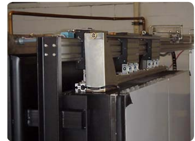
Slide assembly and pneumatic cylinder.
